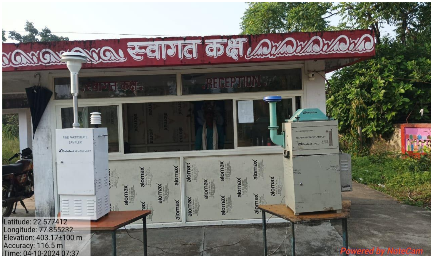
Ambient Air Monitoring near Kendriya Vidyalaya
